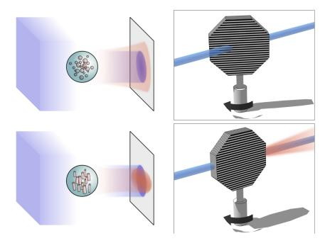
Illustrations of scattering mechanisms used for X-ray dark field imaging. On the left: small angle scattering can be either isotropic or directional depending on the inner structure of a sample. On the right: ordered structures can give rise to a strong scattering signal when they are aligned with the propagation direction of the x-ray beam. This effect can also be used to characterise the inner structure.
