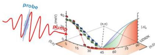
Fig.1 : The idea of the research project proposed is to combine the excitation with long wavelength pump pulses (red) with high frequency short probe pulses (blue). The probe pulses shorter than the wavelength of the pump field will allow for the measurements of responses of the SC with amplitude and phase selectivity. In addition to this (see text), non classical statistical features of the probe pulses will be measured.
